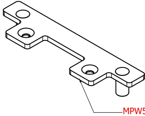
MPW50TBRPA - RAIL RETAINER PLATE (4)
