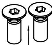
M514FLTXBT - M5 x 14mm TX25 DRIVE BLOCK SCREW (2)
